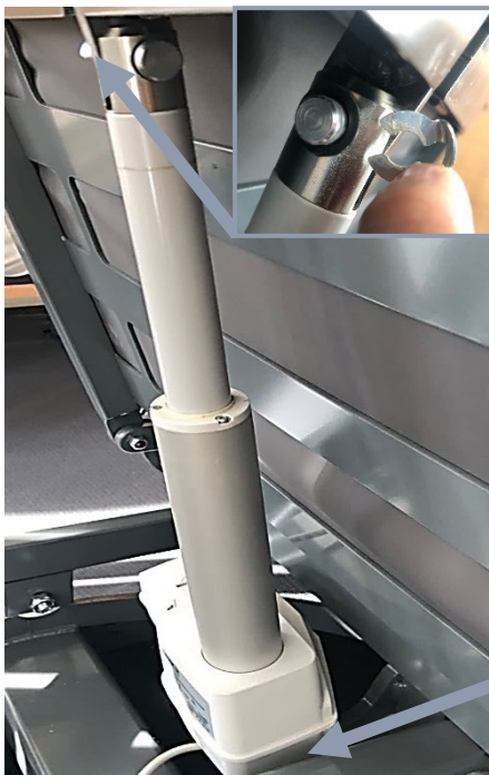
Location of retaining clip and bolt
