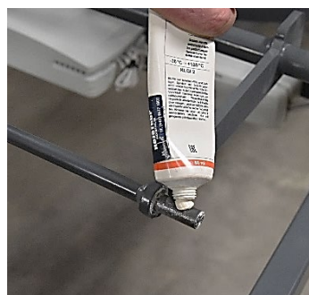
Apply grease on axle
