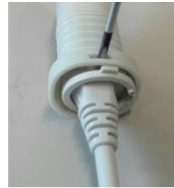
Removing the cable lock using a flat-blade screwdriver
