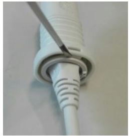
Removing the cable lock using a flat-blade screwdriver
