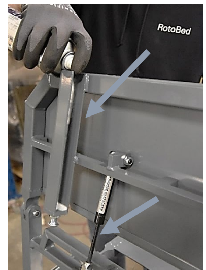
Spray in U-profile and on the thin strut
