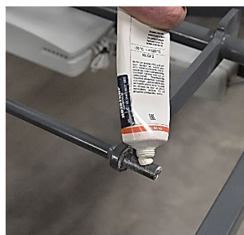
Apply grease on axle
