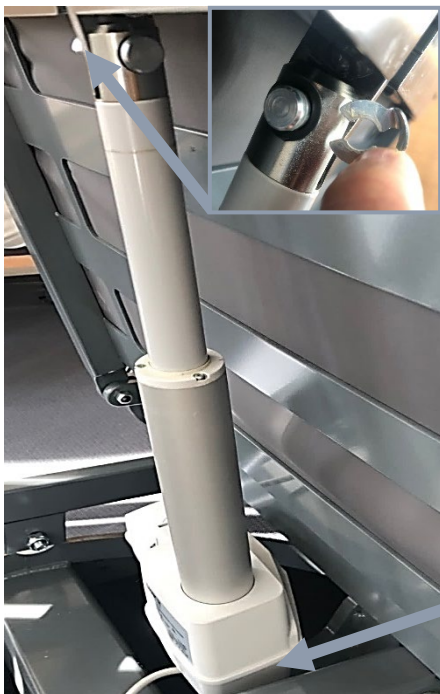
Location of retaining clip and bolt
