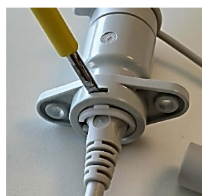
Removing the cable lock using a flat-blade screwdriver
