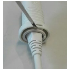
Removing the cable lock using a flat-blade screwdriver
