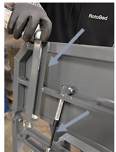
Spray in U-profile and on the thin strut
