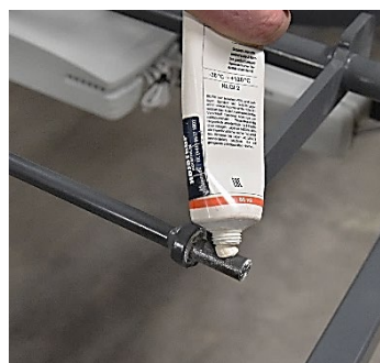
Apply grease on axle
