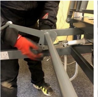
First, mount the new leg motor to the front bracket of the motor and then attach it to the rear bracket. Loosen the nuts on the motor bracket.
