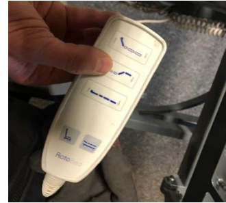
Move the motor to the outer position by holding the "up" button to the foot end inside.
