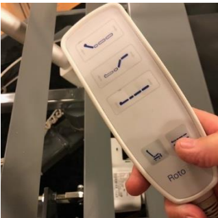
Then press the "lying button" until the motor stops - in this position the distance from the center of the bolt hole to the large cylinder on the leg motor is approx. 10 cm.
